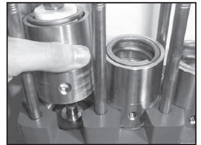
9. Place new plunger pipe (29B) carefully through the oiled seals and push seal sleeve (35) with plunger pipe into the crankcase guide. **Note: Make sure weep hole is facing down.**
