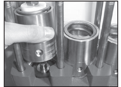
9. Place new plunger pipe (29B) carefully through the oiled seals and push seal sleeve (35) with plunger pipe into the crankcase guide. Note: Make sure weep hole is facing down.
