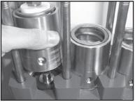
9. Place new plunger pipe (29B) carefully through the oiled seals and push seal sleeve (35) with plunger pipe into the crankcase guide. *Note: Make sure weep hole is facing down.*
