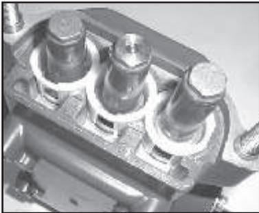
10. Inspect ceramic plunger (24A) tips for wear. If necessary, replacement of the ceramic plungers may be accomplished by removing the plunger bolt assemblies (24) with a 13mm wrench. Ceramic plungers should now slide off the stainless steel plunger base (22). Excessive resistance to plunger removal may be overcome by heating the stainless steel plunger base. This will melt any excess loc-tite beneath the ceramic plunger allowing easy removal.
