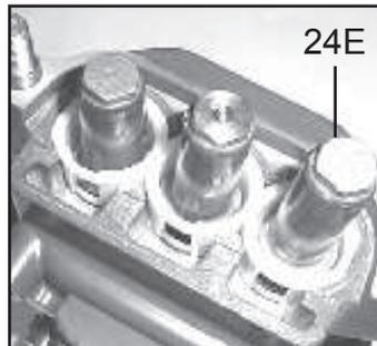
11. Replace copper ring (24E) onto plunger bolt (24B). Slide plunger bolt assembly (24) into ceramic plunger (24A). Apply a light film of loc-tite to plunger bolt threads and place plunger assembly onto stainless steel plunger base (22) and tighten to 310 in.-lbs. (35 Nm).
