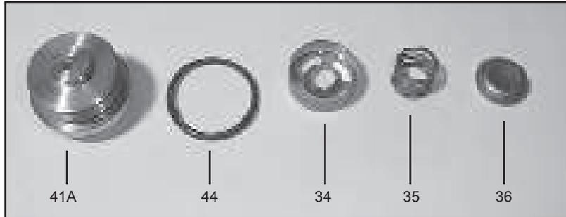
2. Check o-ring (44) for wear and replace as necessary. Remove the discharge spring retainer (34), valve spring (35), and valve plate (36).
