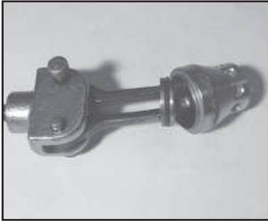
8. With a valve puller remove the valve seat (37) and o-ring (38). If excessive pitting is seen, replace the worn parts. Check valve seat o-ring (38) for wear and replace as necessary.
