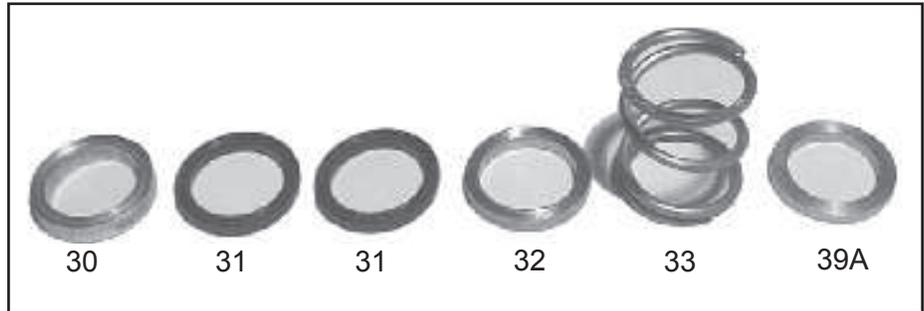
9. Remove the spacer (39A), pressure spring (33), support ring (32), v-sleeves (31), and pressure ring (30), from the manifold (29) and check for wear.
