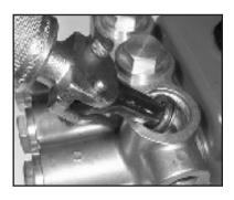
3. Use a small slide hammer to remove valve seats (37) from manifold (29). Inspect valve plate (36) and valve seats (37) for wear. If excessive pitting is seen, replace the worn parts. Check valve seat o-ring (38) for wear and replace as necessary.
