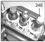
11.Replace copper ring (24E) onto plunger bolt (24B). Slide plunger bolt assembly (24) into ceramic plunger (24A). Apply a light film of loc-tite to plunger bolt threads and place plunger assembly onto stainless steel plunger base (22) and tighten to 310 in.-lbs. (35 Nm).
