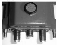
13.Before replacing pump manifold (29), first rotate crankshaft (18) until two outside plungers (24A) extend evenly forward. Lubricate ceramic plungers with a light film of oil. Carefully and evenly slide manifold over plungers and press manifold firmly against crankcase (1). Replace manifold stud bolts (45), washers (47) and nut (46) and tighten to 59 ft.-lbs. (80 Nm).
