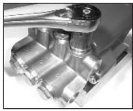
With a 22mm socket, remove the three discharge (43) and three inlet (41) manifold plugs.
