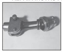
8. With a valve puller remove the valve seat (37) and o-ring (38) replace if worn. If excessive pitting is seen, replace the worn parts. Check valve seat o-ring (38) for wear and replace as necessary.
