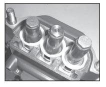
Inspect ceramic plunger (24A) tips for wear. If necessary, replacement of the ceramic plungers may be accomplished by removing the plunger bolt assemblies (24) with a 13mm wrench. Ceramic plungers should now slide off the stainless steel plunger base (22). Excessive resistance to plunger removal may be overcome by heating the stainless steel plunger base. This will melt any excess loc-tite beneath the ceramic plunger allowing easy removal.
