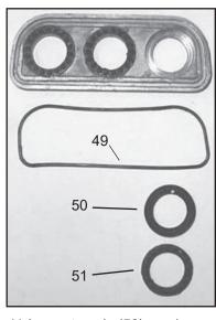
11.Inspect seals (50), seal support ring (51) and O-ring (49) and replace as necessary.
