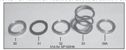
9. Remove the spacer (39A), pressure spring (33), support ring (32 or 31A for SP100HK), v-sleeve (31), and pressure ring (30), from the manifold (29) and check for wear.
