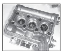
7) Remove the pressure rings (24) and v-sleeves (23) from the valve casing (26).
