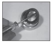
8) Remove the weep grooved seal (23) out of the seal adaptor (20). Check O-rings (21). **IMPORTANT!** The grooved seal (23) on the high-pressure side is to be fitted carefully into the valve casing (26) using a screwdriver. Under no circumstances must the seal surface in the valve casing or the seal lip be damaged.
