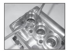
6) Remove seal adaptors (20) and weep return rings (25) from the valve casing.
