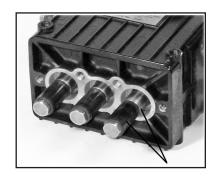
13. Check surfaces of the plunger bases and plunger pipes (#16B). A damaged surface will cause accelerated wear on the seals. Deposits of any kind must be carefully removed from the plunger surface. A damaged plunger must be replaced!
