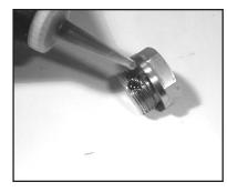
5. Apply one drop of Loctite 243 to valve plugs (32) and tighten to 55 ft.-lbs. (75 Nm). For pumps manufactured prior to 5/97 tighten plugs to 37 ft-lbs. (50 Nm).
