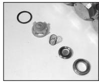
4. Remove each o-ring (#31). Inspect all parts for wear and replace as necessary. Reassemble valve assy's (32X) & place in valve casing (26)
