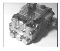
Using a needle nose pliers, remove the inlet and discharge valve assemblies (26A) and o-ring (31). Inspect all parts for wear and replace as necessary.
