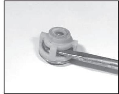
3. By inserting a small screw driver between the valve seat (27) and the valve spring retainer (30), the valve assembly can be separated.
