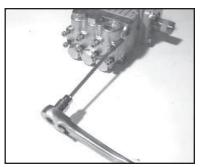
5. Next, use a 5mm allen wrench to remove the eight (8) socket head cap screws (34).
