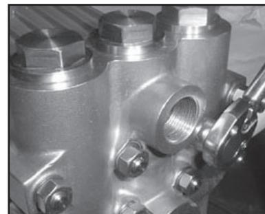
13) Place entire manifold assembly sleeve assembly over the studs (49) and push firmly until seated against the crankcase (1).
