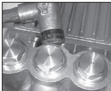
7) If needed, tap valve casing with a rubber mallet to remove it.
