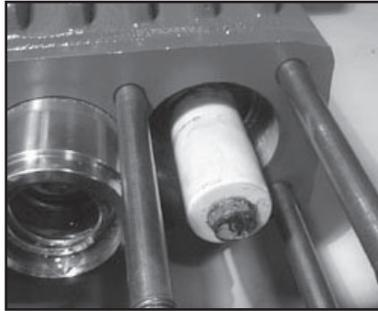
10) Check plunger surface (25 and 29B) and seals (40) for wear and pitting. If none is found, proceed to step twelve.
