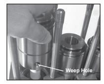
12) Check plunger surface (29B). If plunger pipe is worn out, loosen tension screws (29C) with a 15mm socket and pull off plunger pipe to the front. Clean front surface of plunger (29B) thoroughly. Apply a small drop of locktite to tension screw. Put a **new** crush washer (29D) onto tension screw. Put a thin coat of glue (Loctite) on the ring (or ceramic plunger side) and tighten screw to 265 in.-lbs. (30 NM).
