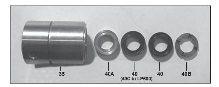
11) Remove the pressure ring (40A), v-sleeves (40), sleeve (40C in LP600 only), and support ring (40B), from the seal sleeve. For LP301A and LP301A-4000 pumps, remove the pressure spring (41). Examine seals carefully and replace if worn. Clean surfaces of seal sleeves (35) which come in contact with the crankcase (1) and sealing surfaces of valve casing (43).
