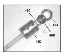
4) Loosen valve seats (46A) and valve spring (46C) from spacer pipe (46D) by lightly hitting the valve plate (46B) with a plastic stick. LP600/LP600-4000 pumps have an additional valve spring guide (46E). Check sealing surface and replace worn parts. Reassemble with new O-rings (44A) if possible and oil them before installing.
