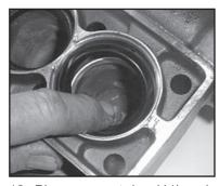
Place support ring (41) and v-sleeves (40) into valve casing. For LP250-3100, the support disc (37) is placed in the manifold (43) before the support ring.
