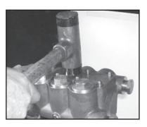
14. Place entire manifold/seal sleeve assembly over the studs (49) and push firmly until seated against the crankcase.
