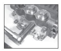
3. Remove the eight (8) hex nuts (49A) with a 19mm wrench. Tap the back of the manifold (43) with a rubber mallet to dislodge and slide off the studs.
