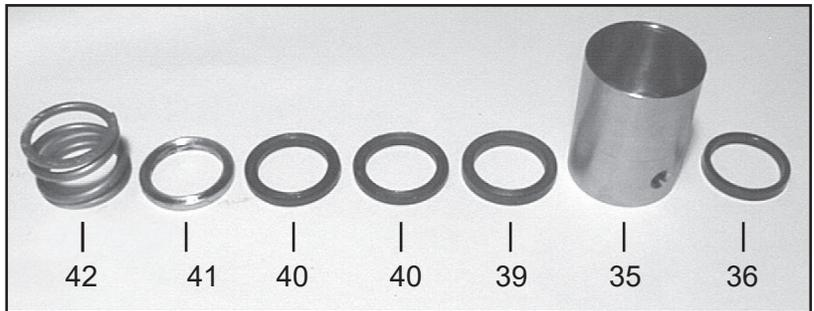
7. Remove the tension spring (42), support ring (41), v-sleeves (40), pressure ring (39), from the seal sleeve (35). Examine seals (36) carefully and replace if worn. Clean all parts.
