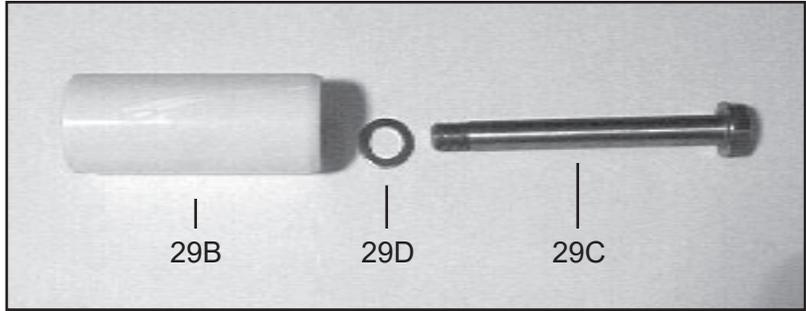
9. Check plunger surface (29B). If plunger pipe is worn, loosen tension screws (29C) and pull off plunger pipe to the front. Clean front surface of plunger (25) thoroughly. Apply a thin coat of Loctite to the tension screw threads (29C). **Note: Care must be taken that no glue gets between the plunger pipe (29B) and the centering sleeve (29A).** Add new copper ring (29D).
