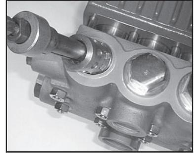
3. Remove the complete valve assembly (46A-46D) with valve pullers.
