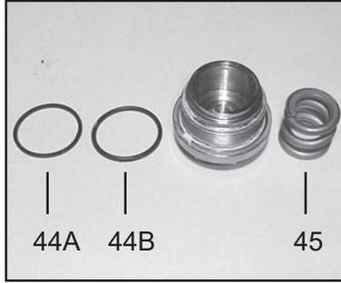
2. Remove the compression spring (45), O-rings and support rings (44A & 44B).
