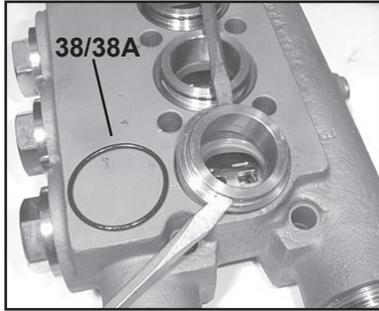
8. Remove seal case (37) from valve casing (43) and inspect O-rings (38/38A).
