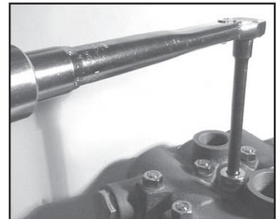
12. Place valve vasing (43) over studs and push firmly until seated against the crankcase (1). Tighten the hexagon nuts (49A) in a crosswise pattern (shown below) to 59 ft.-lbs. (80 NM)
