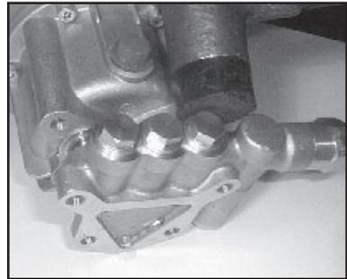
6. Tap the back of the manifold (35) with a rubber mallet to dislodge, and slide off the plungers. (8). Take note of the position of the discharge port so as to place the manifold in the same position during reassembly.
