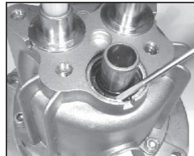
7. Remove the guided p-valve, (19), valve springs (18), v-sleeves (21) and pressure rings (20). Inspect for wear and replace as necessary. Remove the spacer ring (17) from the plungers (8).
