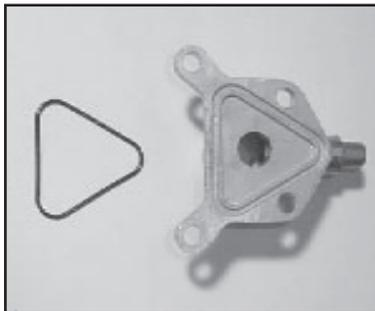
5. Remove the suction flange (39) and flange o-ring (38). Inspect the o-ring for wear and replace as necessary.
