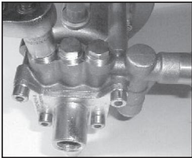
1. With a 14mm socket wrench, remove the three discharge valve plugs (27). Inspect the valve plug o-rings (23) for wear, and replace as necessary.
