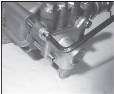
4. Next, remove the four manifold bolts (40) with a 6mm allen wrench.
