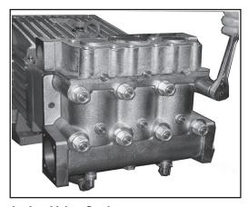
Replacing Valve Casing:
