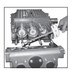
9) Lightly coat the seal sleeve with anti-corrosive grease (e.g. molycote no. Cu-7439) in its fitted area towards the crankcase. Insert the seal sleeves in to their crankcase fittings. Lightly coat the threads of the tension screw (36C) with thread glue and insert it together with a new copper ring (36D) through the ceramic pipe. Turn the pump by hand until the plunger (25) rests against the plunger pipe. Tighten the tension screw at 30 Ft-lbs. (40 Nm).
