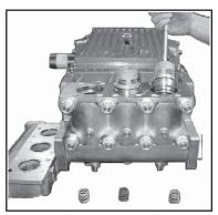
3) Take out pressure springs (57A). Pull out assembled valves (51 & 52) with valve pulling tool (07662).
