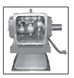
11) Take out plungers and seal sleeves as described above. Drain the oil by taking off the plug (12). After removing the clip ring (33B), pry out the seal retainer (33) with a screwdriver. Open hose adaptor (K11) and remove gear cover (K3) and the cooling vane plate (K1) by removing the screws (K4).
