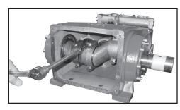
12) Remove the connecting rod screws (24).
