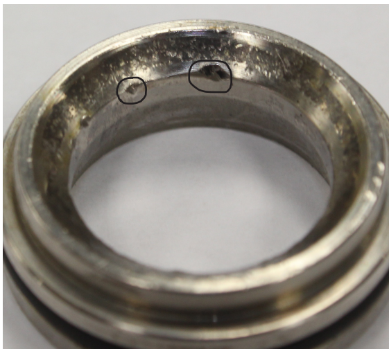
Fig. 1-1. Notice the pitting of the valve seat.
