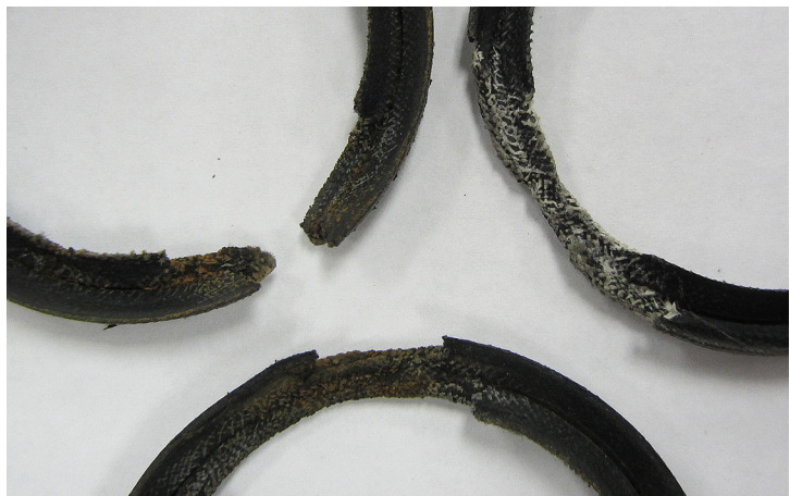
Fig. 1-2. Notice the uneven wear on seals from a cavitating pump.
