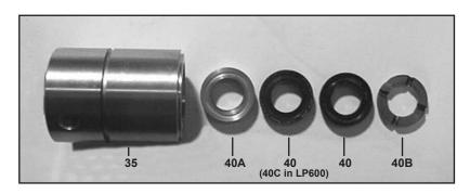
11) Remove the guide ring (40A), v-sleeves (40/40C), and support ring (40B), from the seal sleeve. Examine seals carefully and replace if worn. Clean surfaces of seal sleeves (35) which come in contact with the crankcase (1) and sealing surfaces of valve casing (43).
