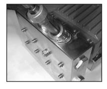
3) Take out discharge valve assemblies (46) by pulling them upwards out of the valve casing (43) with a snap-ring tongs or any other pull-off device. Then remove inlet valves in the same way.
